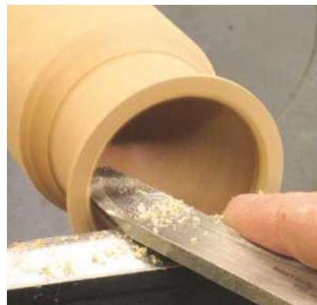
▲ Pic.12 The tool is presented horizontal on the rest and cutting on the centreline. To achieve the best finish remove only small amounts of timber and keep the tool on the move
